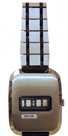
Figure 50 – very early LCD watch with "random dispersal" display
