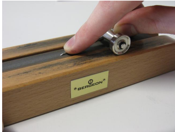
Figure 109 – using a screwdriver sharpening device
