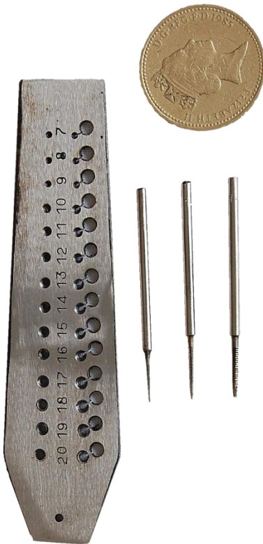
Figure 134 – screw plate and three watch-sized taps, with a pound coin for scale
