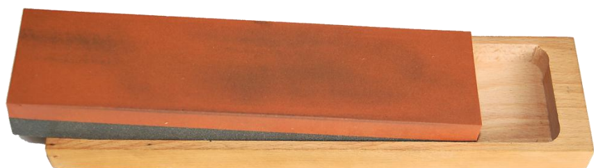
Figure 135 – India (aluminium oxide) stone
