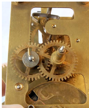
Figure 60 – motion work on the front of the clock
