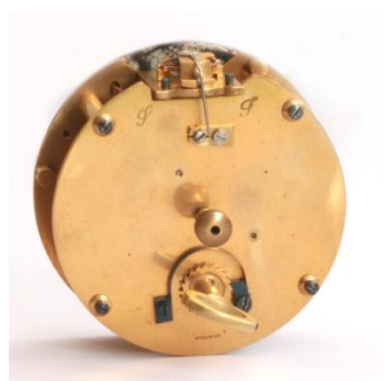
Figure 20 – drum movement showing platform escapement
