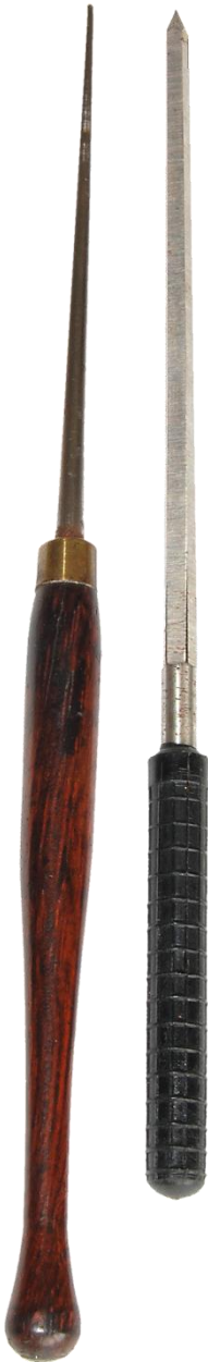
Figure 131 – smoothing broach (left), and cutting broach
