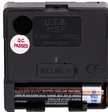
Figure 42 – radio controlled quartz movement
