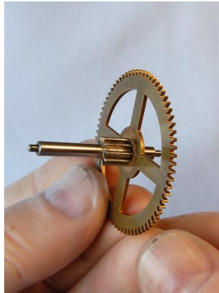
Figure 85 – intermediate wheel and pinion
