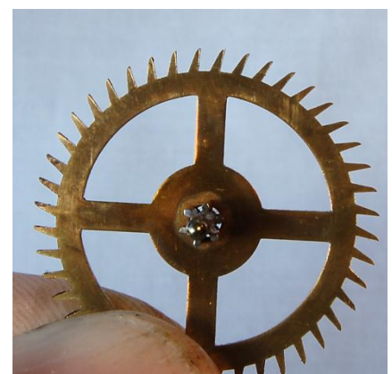
Figure 88 – tooth form of escape wheel
