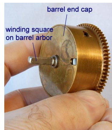
Figure 83 – another view of the barrel
