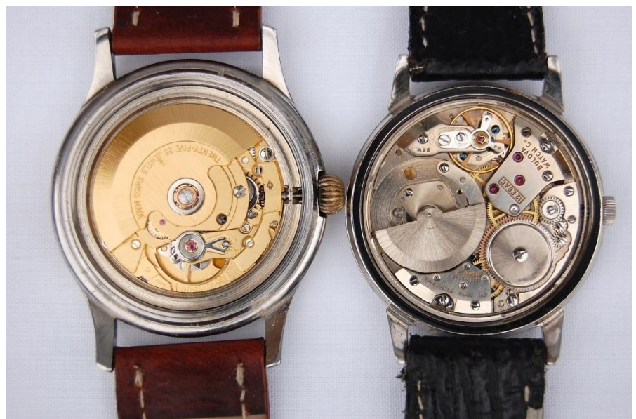
Figure 47 – 20th century ETA and Bulova movements
