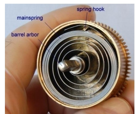
Figure 84 – barrel with end cap removed
