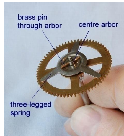
Figure 90 – the components of the friction drive
