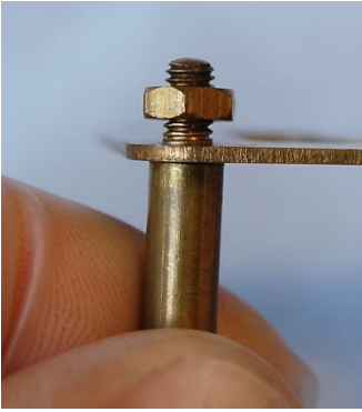
Figure 98 – pillars fastened to plates with nuts
