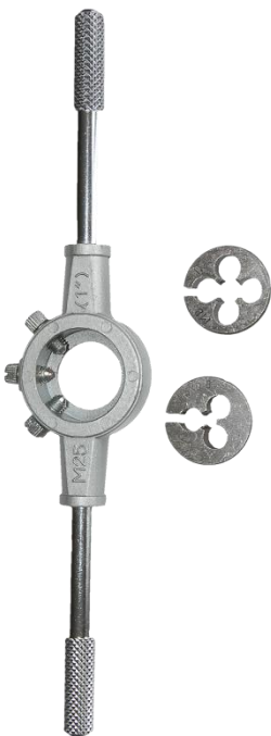
Figure 133 – die stock and two dies
